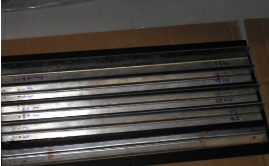
Figure 11: The holes were marked on both the L's and the black aluminum so when more drilling and riveting occurred the holes would be in the right places.
