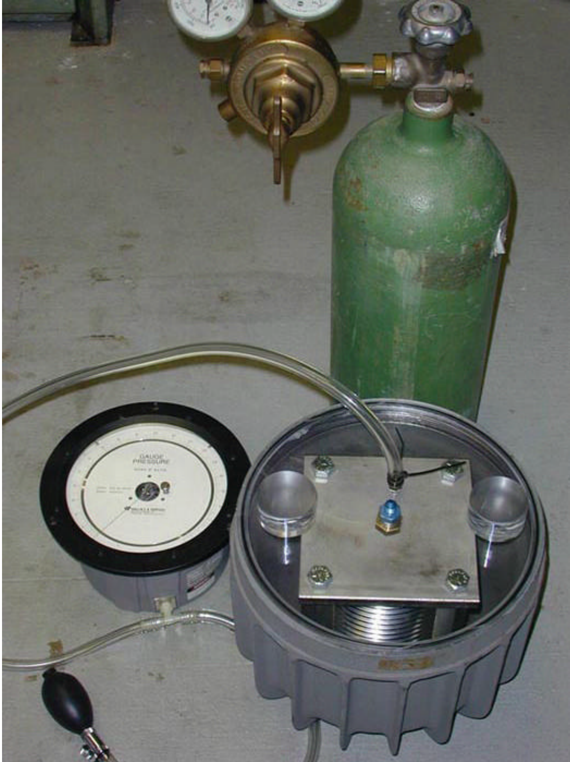
Figure 4: Test assembly filled with water and placed in an enclosed container which is 95% filled with water
