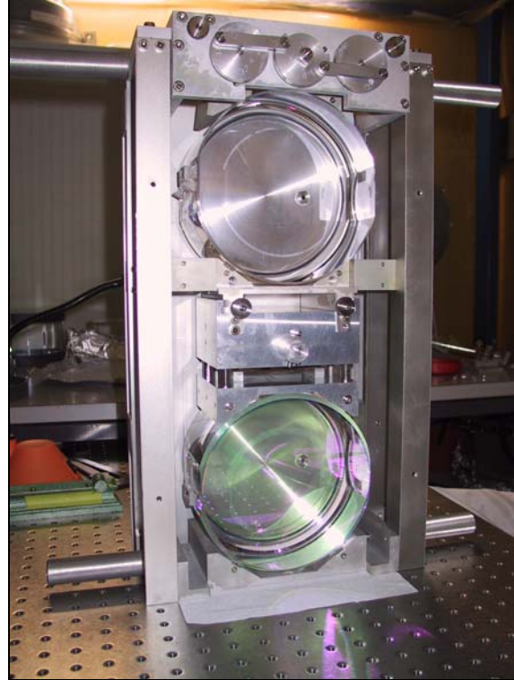
Picture (1 and 2): Picture 1 on the LHS shows one of the main suspensions in GEO 600. Suspended coils can be seen in the aluminum mass in the top left hand side of the picture. Picture 2 on the RHS shows two fused-silica masses in a GEO 600 style catcher / fixture prior to installation into one of tanks.
