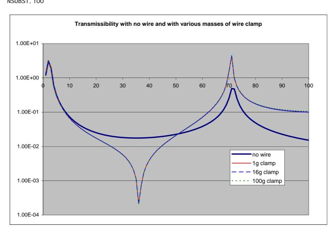
The transmissibility numbers are slightly different for the different clamp masses but no enough to show on the graph. So (partly to check I really have changed the model!) here are the percentage changes 16g/1g ad 100/1g:
