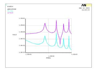
For completeness here is the 1-100 Hz plot repeated for damping ratios of 1e-1,1e-2,1e-3, 1e-4.
