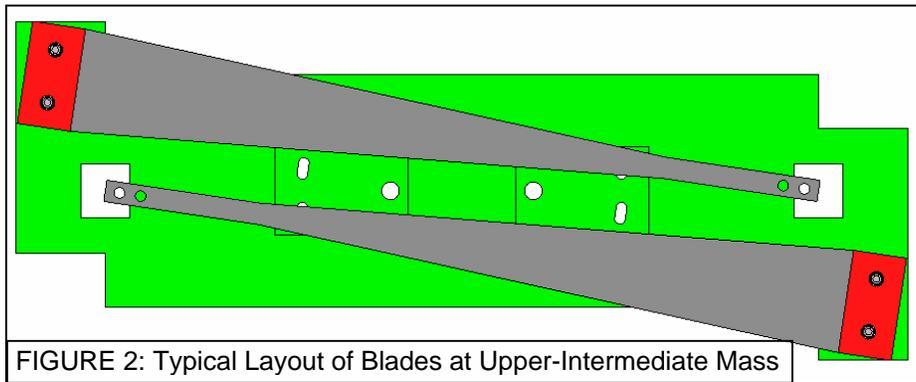
FIGURE 2: Typical Layout of Blades at Upper-Intermediate Mass
