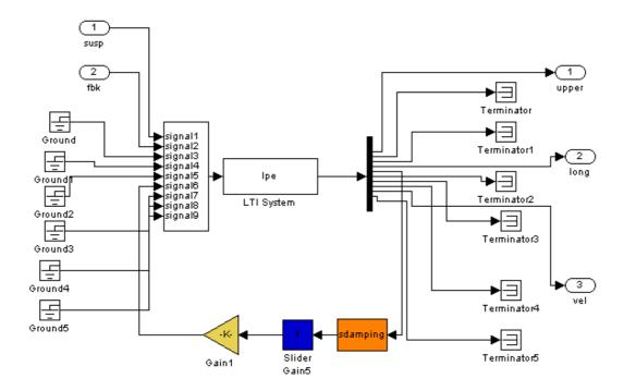
The orange box "sdamping" is the standard local4s.m damping used in earlier models, just to keep pitch modes from complicating the analysis (I don't think this is cheating).
