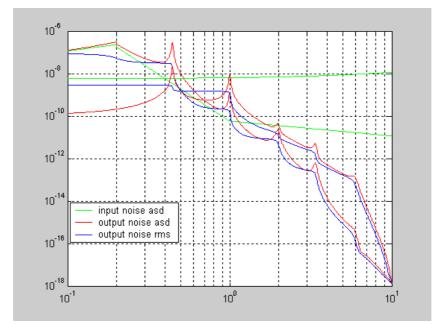
Green curves show the input noise (SEI falls steeper) red curves show mirror velocity amplitude spectral density, and blue curves show that integrated from the right to the left.
