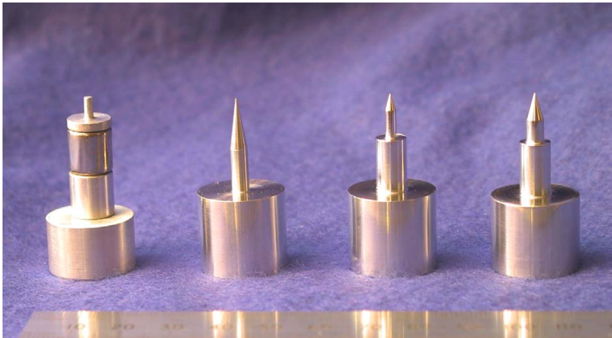
Figure 1. From the left: 2 mm dia. 5 mm long LIGO hybrid OSEM Flag (uppermost part of stack), a 4 mm dia. Flag with a 1:6 taper, and a 2.5 mm and a 4.0 mm dia. Flag, both with a 1:3 taper. A spherical-ended 3.25 mm dia. Flag (not shown) has also been machined. This has been used for the measurements on the twelve different emitter-detector pairs, described below in Tables 3(a) and (b).
