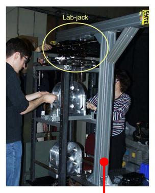
NOTE: Construction of a 'gallows' structure (incorporating a lab-jack to interface with/lift the UI mass) adjacent to the 3&1 Assembly setup
