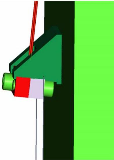
The wire clamp would need good contact with the nose. To get this an indium layer could potentially be added but this would require careful investigation.
