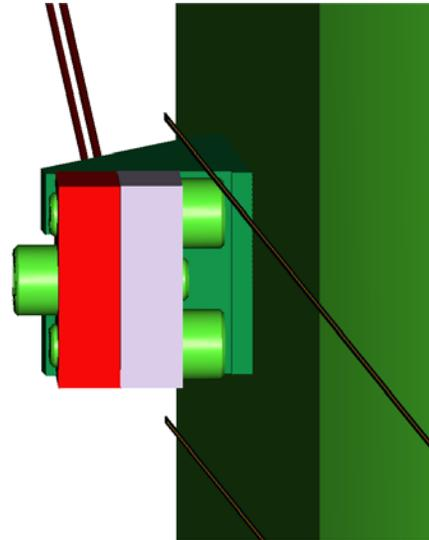
From beneath it is evident that the bolt heads have to be staggered to keep the wire clamp as small as possible. This arrangement maximizes the space around the ribbons.
