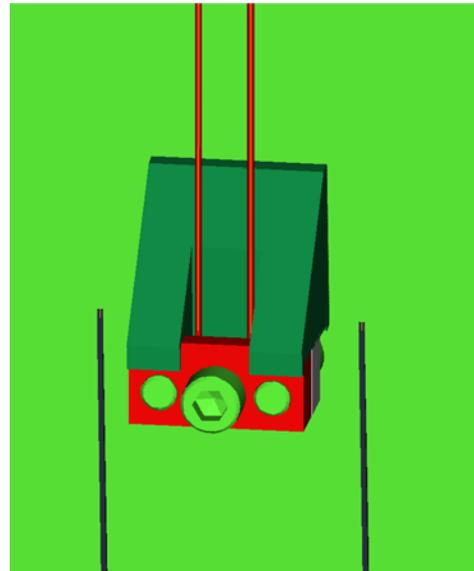
The wire clamp has a knobble on the outer jaw (the red one) which keys into the nose. This prevents slippage in x. Note the ribbons in this model terminate in space.
