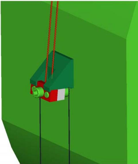
The red and grey wire clamp accommodates the two steel wires (also red) from above. The wire clamp then sits beneath the nose (dark green), and the ledge on the end of the nose prevents slippage in y
