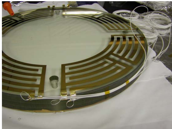
Figure (4): - Photograph of the wiring on the face plate, LIGO-D040052.
