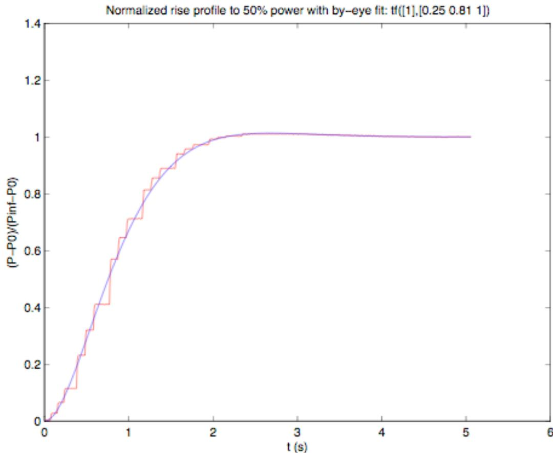
**Figure 6: Transient response of power meter to step power input.**
