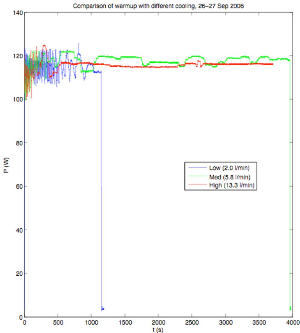
Figure 3: Warm-up profiles - 95% power; 2.0, 5.6 and 13.3 l/min water flow
