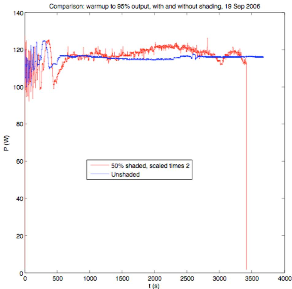
**Figure 4: Warm-up profile – 95% power, with and without 50% beam shading. The 50% curve has been multiplied by 2 to allow easy comparison of relative stability.**
