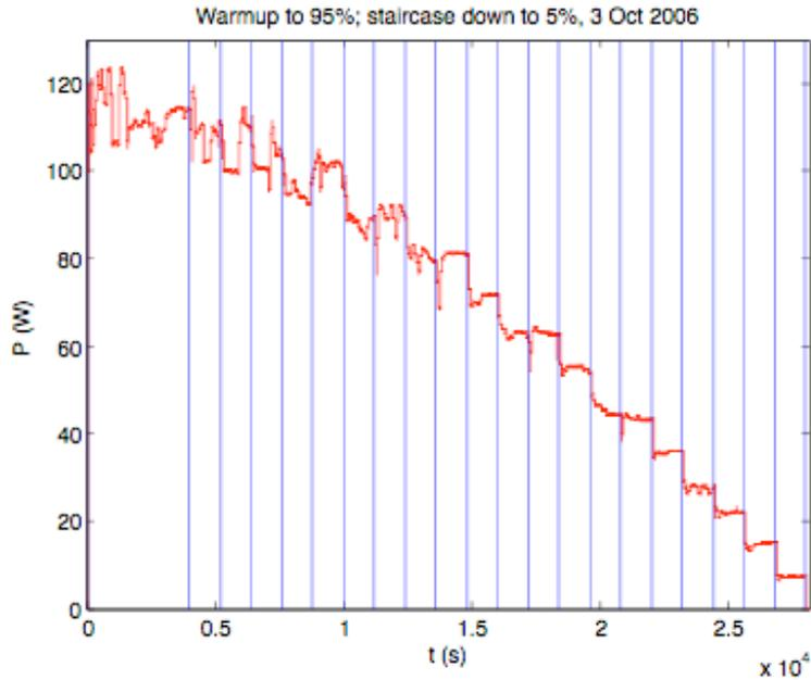
**Figure 5: Effect of repeated negative step functions (nominally 5 W each, or approx 4.5% duty cycle)**
