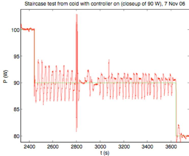
Figure 13: Closeup of apparent instability at 90 W setpoint
