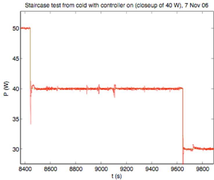
**Figure 12: Closeup of 40 W setpoint tracking**
