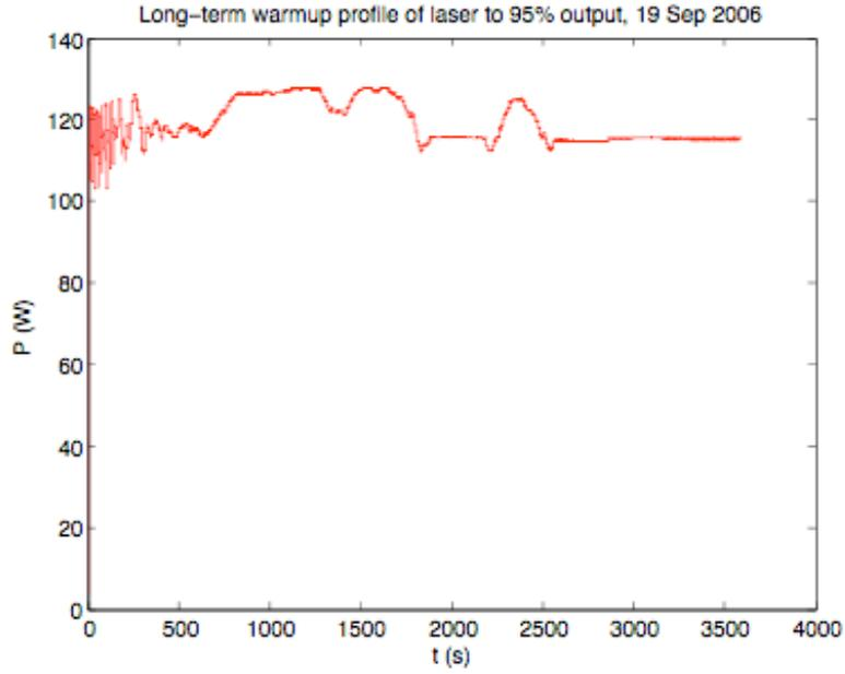
**Figure 1: Warm-up profile of laser – 95% power**
