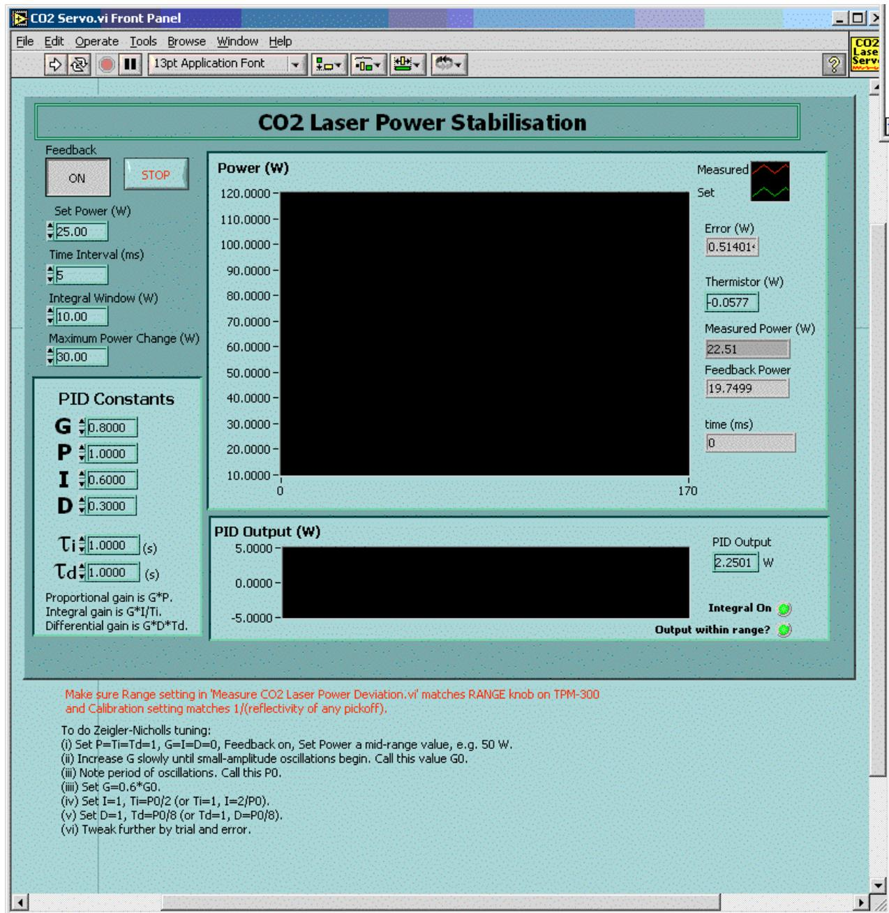
Figure 9: Controller VI main screen
