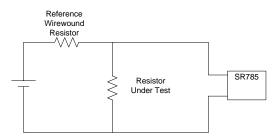
Measurements were made using both a 9V battery and two 9V batteries in series, corresponding to 4.5V and 9V across the test resistor. The input of the SR785 was AC coupled and the range of the instrument was the same for all measurements.
