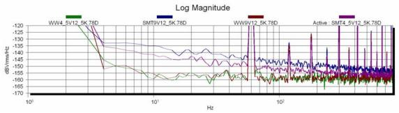
The measurement results for the 1Kohm wirewound and thick film SMT resistors are shown in curves below.
