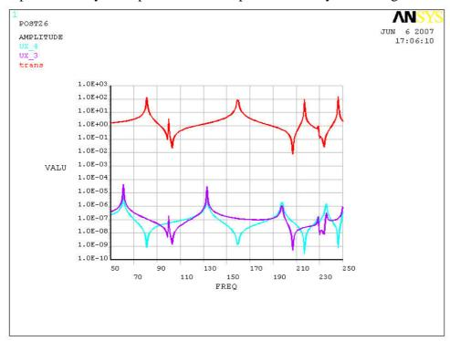
The blue curve is the motion at the input point, the purple curve is motion at the output point, the red curve is transmissibility (which agrees with the previous result).
