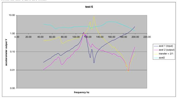
The ink and blue curves are the accelerometer signals by the input" and "output" points on the ET structure – the yellow curve is transmissibility. The light blue curve is the frequency-response of the exciter taken with no load connected.
