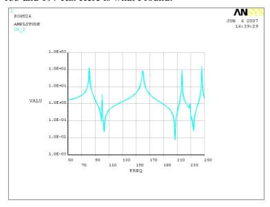
The identifiable features reflect the normal modes of the model with a constraint at the input point.
