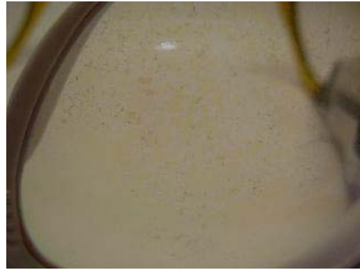
Figure 3. The Uvex LC542 C739 laser safety eyewear that was used at the 40m Lab. On the right is a close-up view of the damaged coating region.
