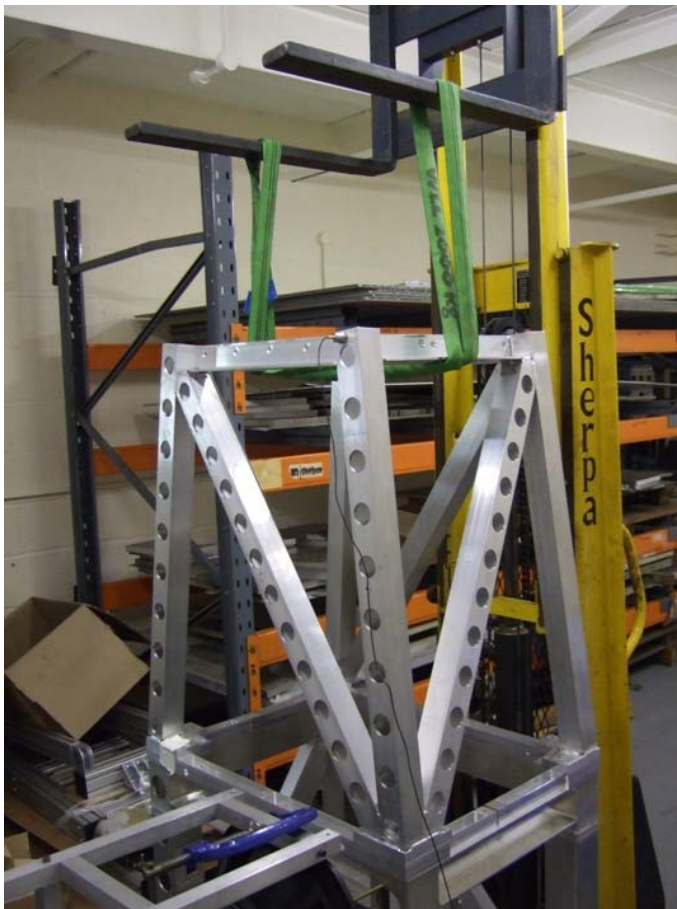
Fig 4. An accelerometer is positioned on the front face of the upper structure in the bottom right corner, as shown in the photograph, this represents channel one.
