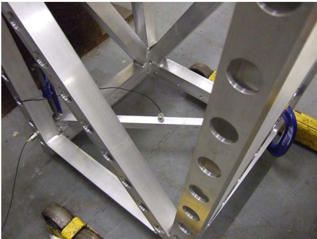
Fig 15. Accelerometer placed mid-span of the square bar
