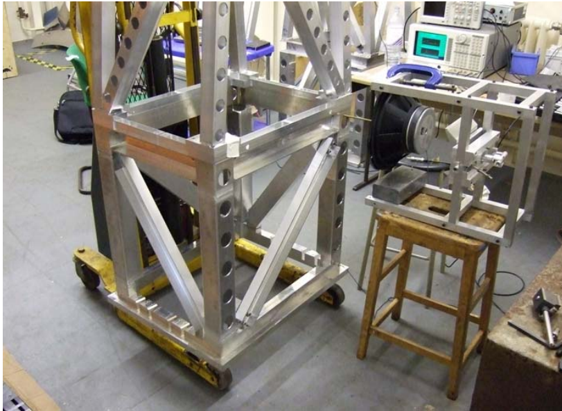
Fig 4. An accelerometer is positioned on the front face of the upper structure in the bottom right corner, as shown in the photograph, this represents channel one.
