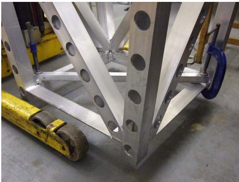
Fig 13. A square bar clamped across the corners of the sleeve structure.
