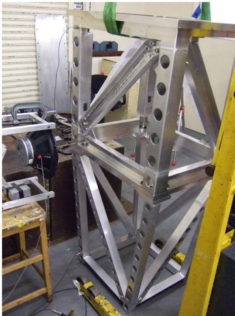
Fig 10. The upper and sleeve structure suspended at the upper structure end by a sling.
