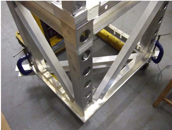
Fig 7. Channel section clamped across the corners of the upper structure.
