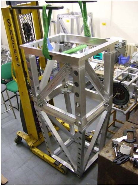
Fig 10. The upper and sleeve structure suspended at the upper structure end by a sling.
