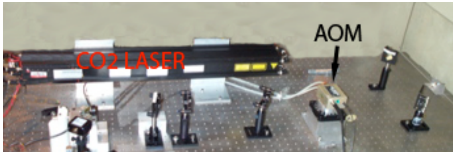
Figure 5. Photo of CO2 laser and AOM in setup for photodiode measurement.
