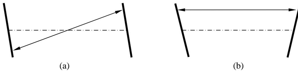
Figure 1: Two different resonator configuration (a) stable (b) unstable
