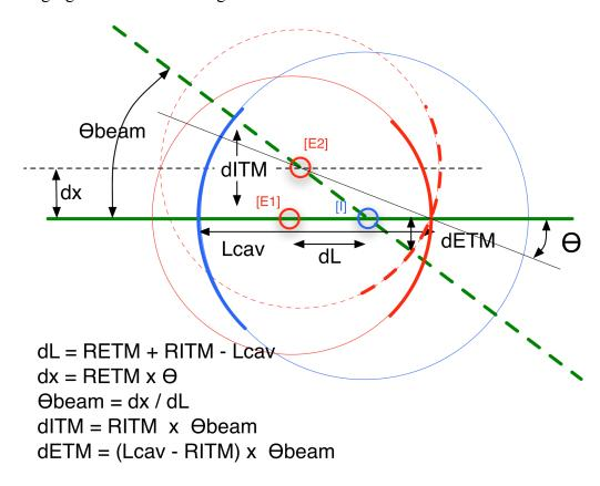
Figure 1 Geometry of mirror tilts and resonating cavity beam
