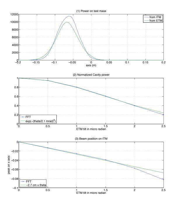
Figure 2 FFT simulation of a FP cavity with tilted ETM
