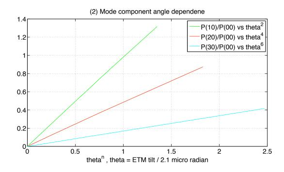
Figure 3 Mode components as a function of ETM angle
