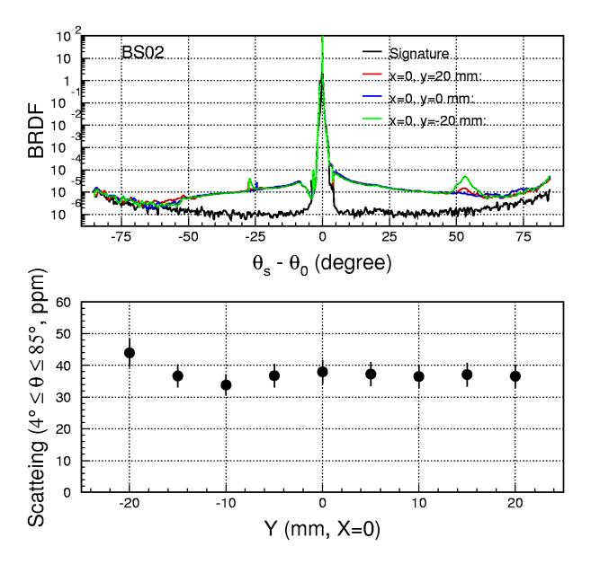
Total nine angular resolved scans are taken along the Y axis with a step of 5 mm, three of them are shown in the upper plot of above figure. The BRDFs of the nine scans are quit consistent, indicating a good uniformity of substrate bulk and AR and HR coatings in terms of scattering. The lower plot shows the integrated scatterings from 4° to 85° polar angle ( $\Theta_s$ -  $\Theta_0$ ) as function of the measurement position.
