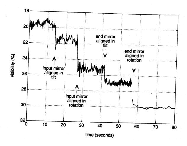
Figure 4: Effect of the automatic alignment system on the fringe visibility of the 10 m cavity.
