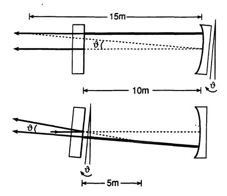
Figure 1: The effects of misalignment of the two mirrors in the plane/curved cavity used for the tests. The directly reflected and cavity leakage beams are indicated schematically by the arrowed lines. (The incident beam in each case is propagating horizontally and strikes the plane mirror at its midpoint.) Note that the path followed by the superposition of the two components depends on their relative magnitudes.
