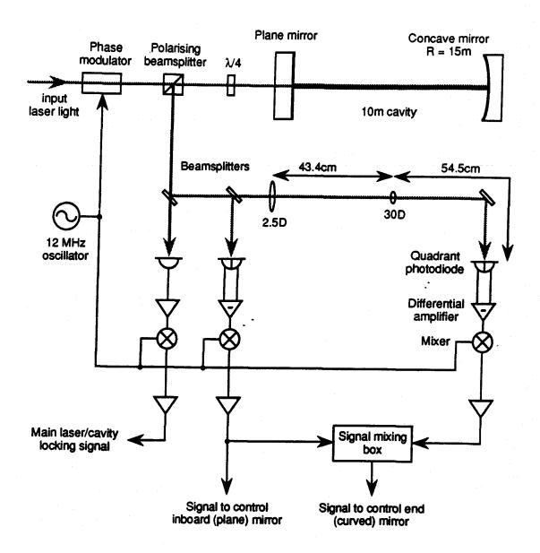
Figure 2: Schematic layout of 10 m suspended optical cavity and the main elements of the control system used for auto alignment in one dimension.
