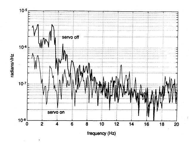
Figure 5: Angular fluctuations as viewed by the sensing system used to control the tilt of the curved mirror in the 10 m cavity.
