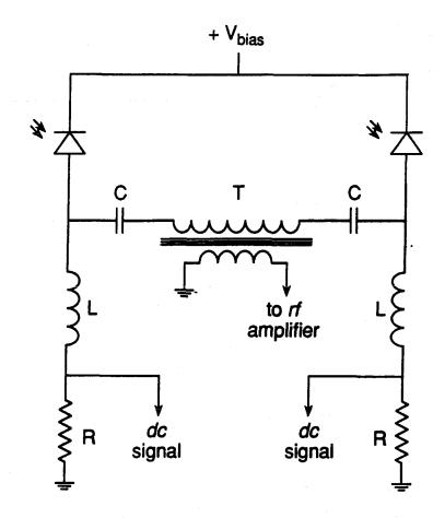
Figure 3: Schematic diagram showing a tuned photodiode front-end for one dimension.
