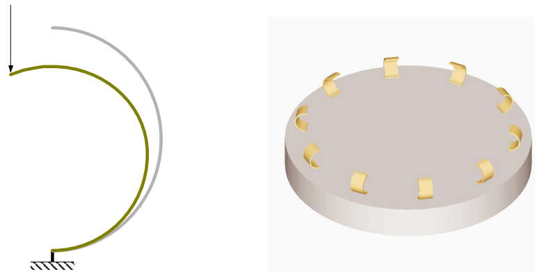
Figure 16: asymmetric deflection of unrestrained leaf spring and spring arrangement to prevent it .
