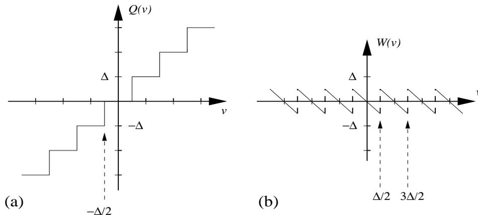
FIG. 2. (a) The quantization function  $Q(v)$  which maps the analog signal into integer multiples of  $\Delta$ , the quantization level, by rounding. (b) The error function which is defined as  $W(v) = Q(v) - v$ .
