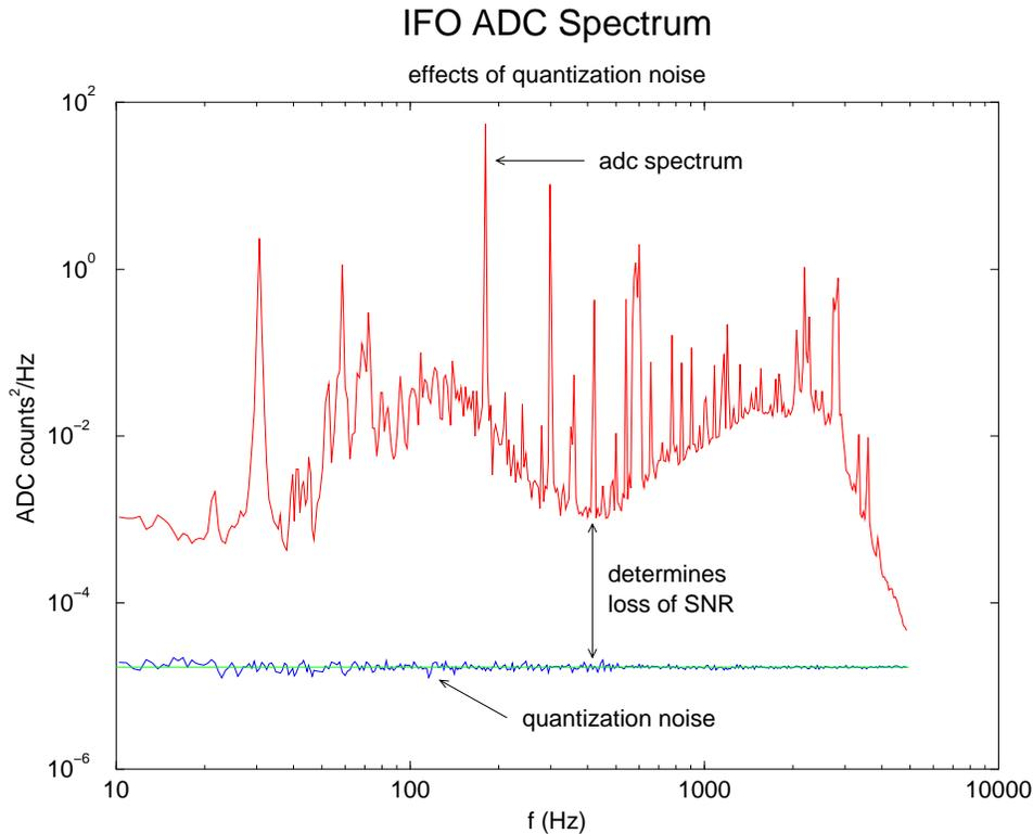
FIG. 1. The IFO power spectrum in  $(\text{ADC counts})^2/\text{Hz}$  is shown in red. This may be compared to the expected spectrum of quantization error  $\Delta^2/12f_N$  shown in green. The expected level of quantization noise was also simulated by replacing the IFO output with uniformly distributed random numbers on the interval  $(-\Delta/2, \Delta/2)$ , shown in blue. The ratio of the powers at the indicated point determines our upper bound on the fractional loss in signal to noise ratio.
