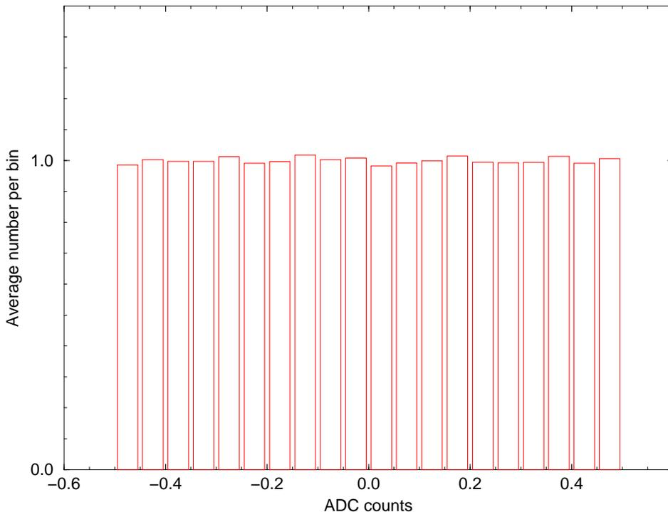
FIG. 4. Simulated Gaussian noise, with the power spectral density of the 40m prototype was quantized as describe above with  $\Delta = 1$ . The quantization noise from 131072 samples was binned into 20 bins in the range  $(-0.5, 0.5]$ , and averaged (divided by  $131072/20$ ). The results shows that this noise is indeed uniformly distributed throughout the interval.
