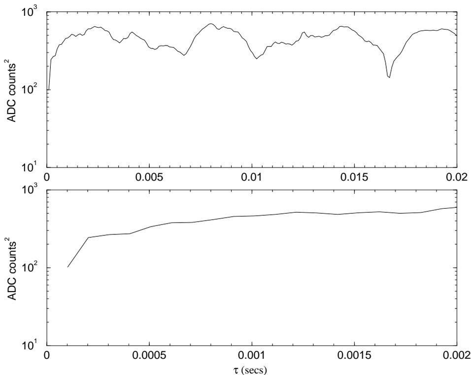
FIG. 3. The function  $f(\tau) = \langle (v(t) - v(t+\tau))^2 \rangle$  in units of  $(\text{ADC counts})^2$  for a quiet stretch of data from the prototype 40m interferometer. The lower graph is zoomed in by a factor of 10 on the upper graph. It is clear that the condition in Eq. (3.6), with  $\Delta = 1.0$  is well satisfied even at for  $\tau = (2f_N)^{-1} \approx 10^{-4}$  sec .
