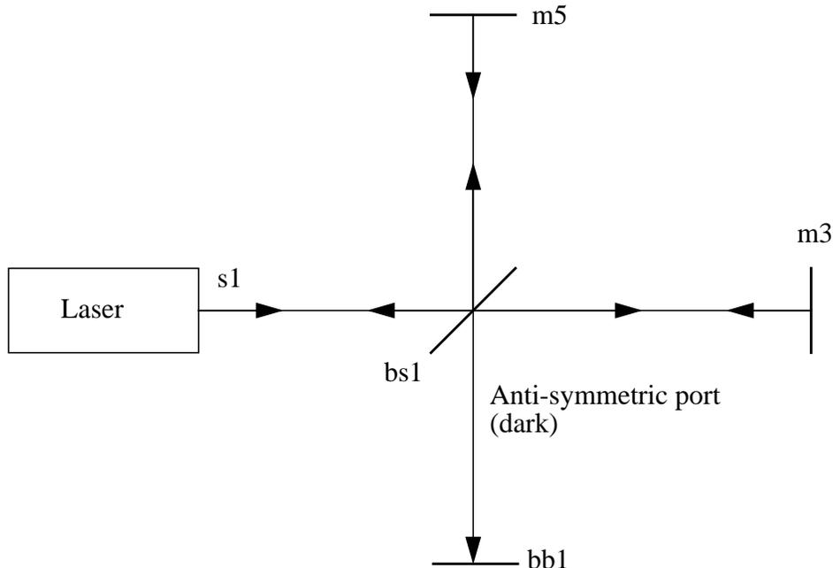
We've had to add a "beam dump" at the antisymmetric port, which is simply an end mirror with 0 reflectivity, which allows us to make a connection to the beamsplitter from the antisymmetric port. *twiddle* will issue an error message if it encounters an interferometer with un-connected inputs.
