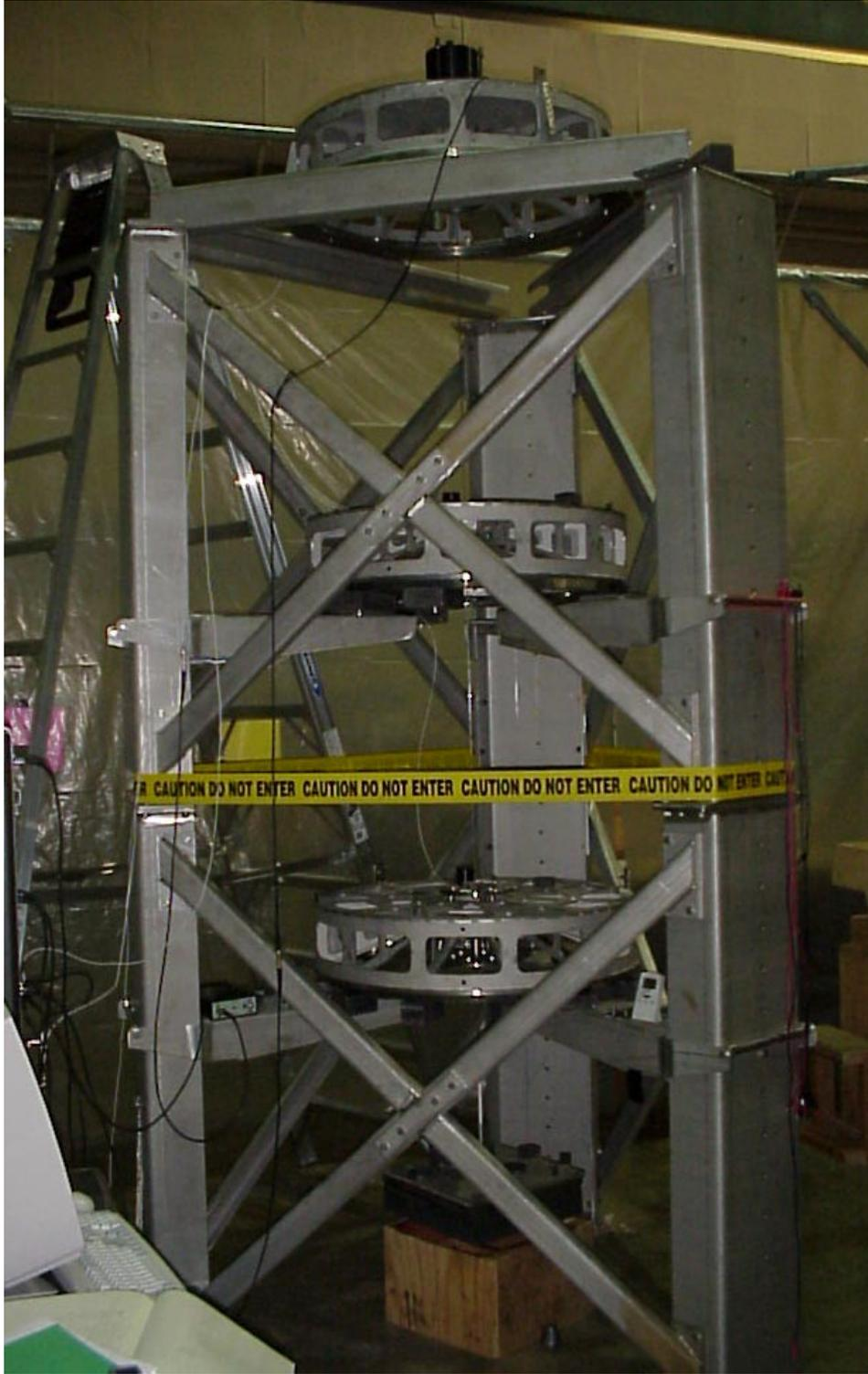
Figure 9: Picture of the actual triple GAS filter chain prototype.
