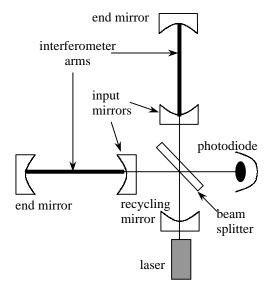
passing gravity wave, a signal would appear in the normally dark side of the apparatus.
