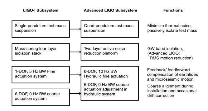
Seismic isolation functions in LIGO-I and Advanced LIGO. (The pendulum suspension, though not part of SEI, is shown because it contributes significant seismic isolation.)
