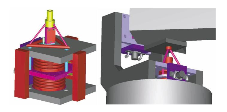
Hydraulic actuator will provide  $\pm 1$  mm, 2 Hz BW continuous actuation in 6 DOF. Each bellows assembly acts in 1 DOF; two DOF at each corner. Viscous fluid and remote pump assure quiet operation.
