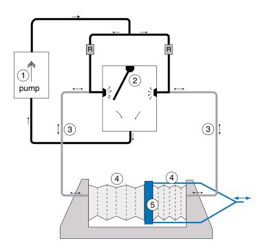
The control valve creates a pressure differential on the bellows. The middle plate is attached with flexures to both the base and the payload, only constraining motion in 1 DOF.
