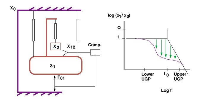
Active seismic isolation.
