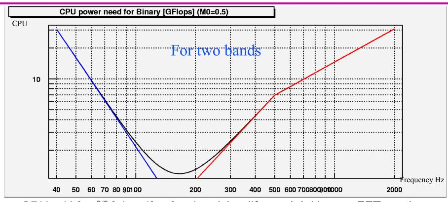
$CPU = K f_{min}^{-8/3} f_{s} log_{2}(f_{min} f_{max})$  (simplify model:  $N_{template}$ .FFT cost)
