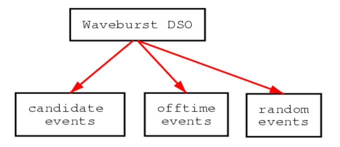
In a single run waveburst DSO is producing 3 kind of events: gw candidate events, offtime events (pixel swapping), random events (pixel mixing).
