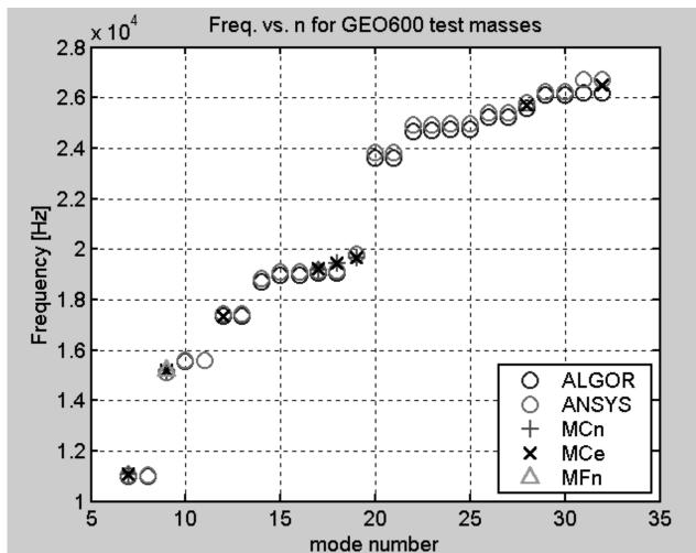
• Mode shapes, freq's determined using ALGOR. Cross-checked using ANSYS (Jena).
