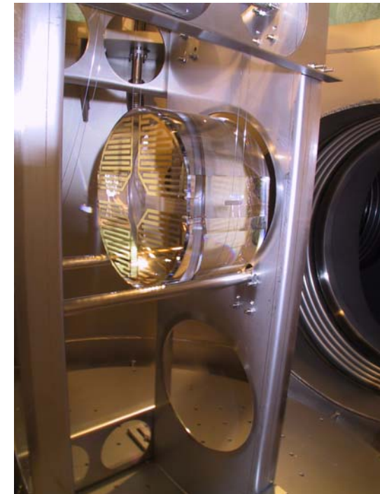
Reaction mass with gold plated grid for electrostatic control
