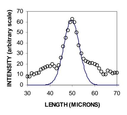
Of all the tested substances, the minimum size of a self-focusing point is in benzene, i.e. 5  $\mu$ m at the length of a nonlinear cell of 60 cm, which results in the precision of wave front inclination measurements  $\lambda/3000$ .
