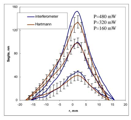
Wavefront distribution when a sample made of BK7 glass was heated by a CO<sub>2</sub> laser beam with different power
