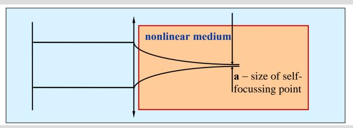
How to get  $\lambda/1000$ ? Use self-focusing to decrease the size of the focal spot. At  $P=P_{critical}$  a  $\rightarrow 0$  and is determined by nonlinear medium properties
