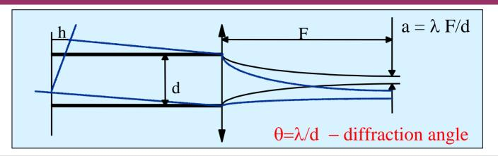
In linear electrodynamics the major limitation to measure wave front deviations angles comes from a finite size of the focal spot .  $h=\lambda/100$  is achieved by an accurate measurement of the transverse beam distribution
