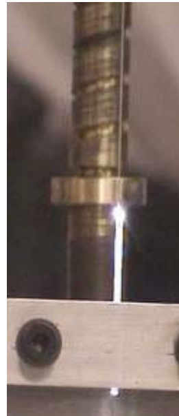
250 \mu\text{m} fibre being pulled using feed & pull technique with CO 2 laser
