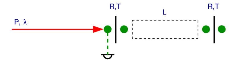
Simple cavity: two mirrors + one space (4 nodes)
