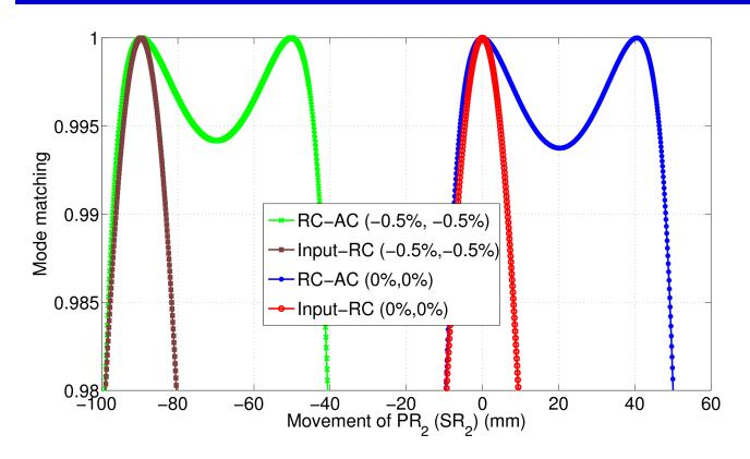
Mode matching betw. Rec. Cavity, Arm Cavity, and Input Mode:
