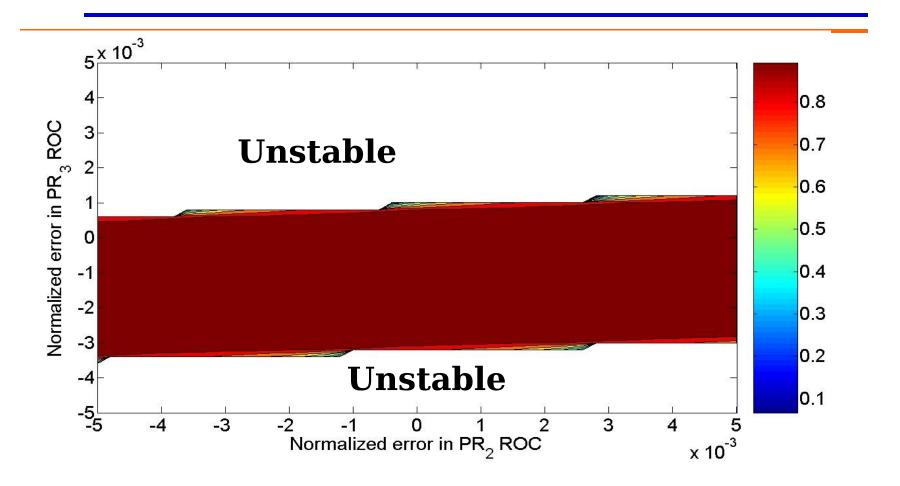
Mode matching between Recycling Cavity and Arm Cavity:
