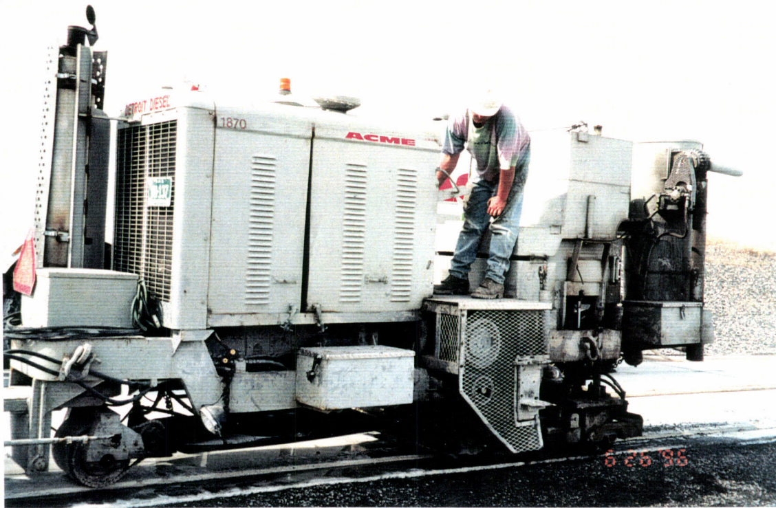
Grinding equipment used to verify the proper elevation of the alignment grooves along both arms.
