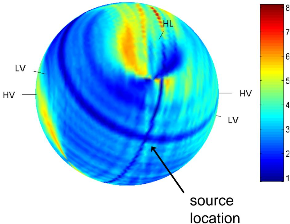
Null energy  $E_{\text{null}}$  varies slowly along rings of constant time delay with respect to any detector pair.
