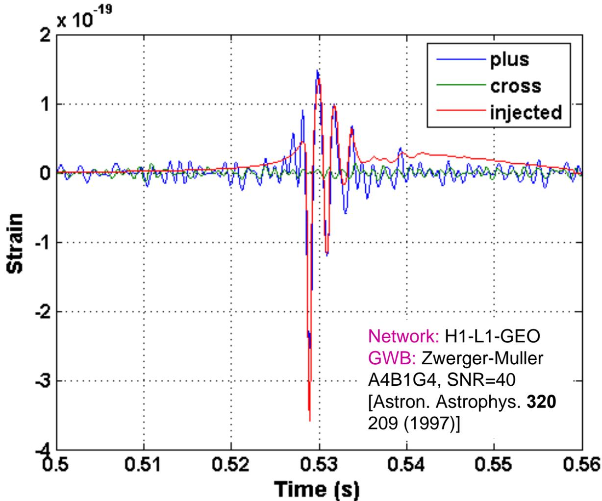
Recovered signal (blue) is a noisy, band-passed version of injected GWB signal (red)
