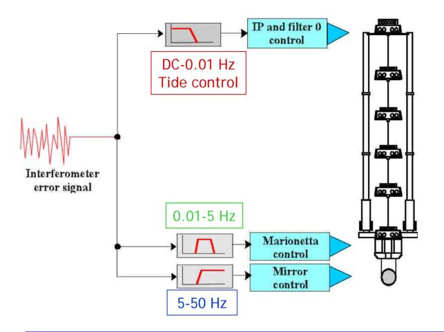
1. Force reallocation over three actuation stages. Allows strong reduction of the force exerted on the mirror
