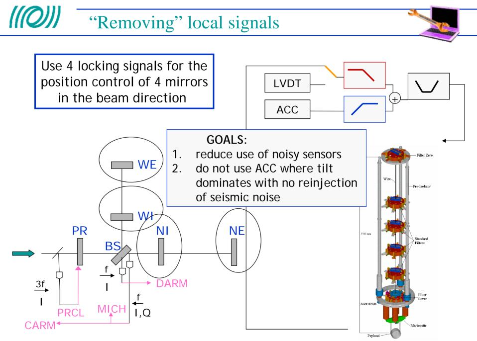
Extending the detection bandwidth down to 10 Hz is a hard job Control noise reduction is a crucial issue
