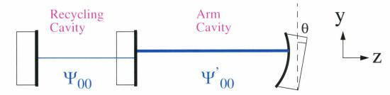
$\implies$  Arm axis is displaced by  $R \theta$  from input axis
