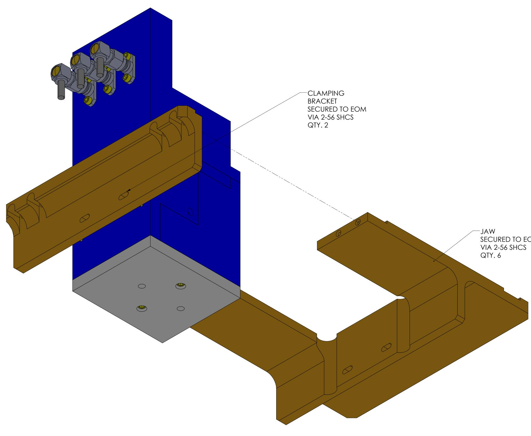
–JAW SECURED TO EOM AND TO CLAMPING BRACKET VIA 2-56 SHCS QTY. 6
