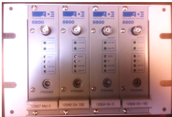
Rack - front view with 4 Gauges inserted
