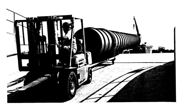
Transporting 22D Beam Tube Assembly to QT Assembly Area
