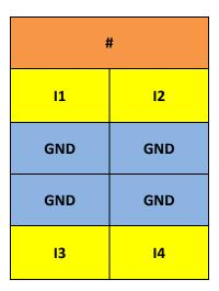
Figure 19: Labels for the 4-channel TTL digital input terminal EL1094.
