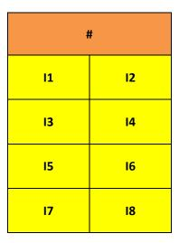
Figure 20: Labels for the 8-channel TTL digital input terminal EL1098.
