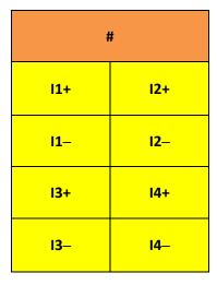
Figure 10: Labels for the 4-channel 16 bit analog input terminal EL3104.
