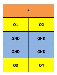
Figure 23: Labels for the 4-channel TTL digital output terminal EL2004.
