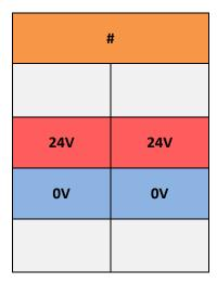
Figure 8: Labels for 24V power supply terminal.
