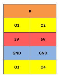
Figure 21: Labels for the 4-channel TTL digital output terminal EL2124.
