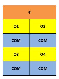
Figure 14: Labels for the 4-channel 16 bit analog output terminal EL4104.
