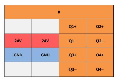
Figure 26: Labels for the 4-channel safety digital output terminal EL2904.
