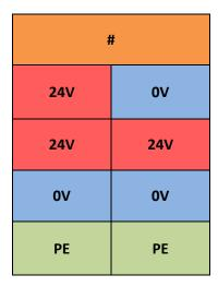
Figure 6: Labels for 24V power supply terminal.
