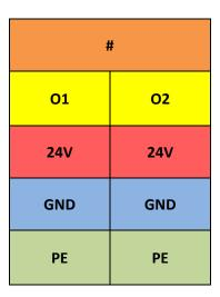
Figure 22: Labels for the 2-channel TTL digital output terminal EL2002.
