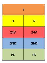
Figure 16: Labels for the 2-channel TTL digital input terminal EL1012.
