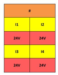
Figure 13: Labels for the 4-channel 16 bit 4...20mA analog input terminal EL3154.
