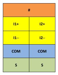
Figure 9: Labels for the 2-channel 16 bit analog input terminal EL3102.
