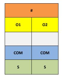
Figure 14: Labels for the 2-channel 16 bit analog output terminal EL4102.
