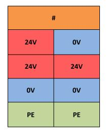
Figure 6: Labels for 24V power supply terminal.
