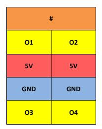
Figure 22: Labels for the 4-channel TTL digital output terminal EL2124.
