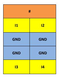
Figure 20: Labels for the 4-channel 24V digital input terminal EL1094 (switching to negative potential).
