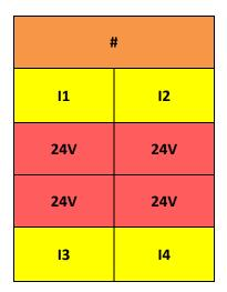
Figure 18: Labels for the 4-channel 24V digital input terminal EL1014.
