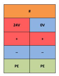
Figure 3: Labels for EtherCAT couplers.
