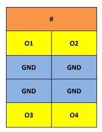
Figure 24: Labels for the 4-channel TTL digital output terminal EL2004.
