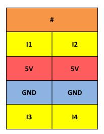
Figure 16: Labels for the 4-channel TTL digital input terminal EL1124.
