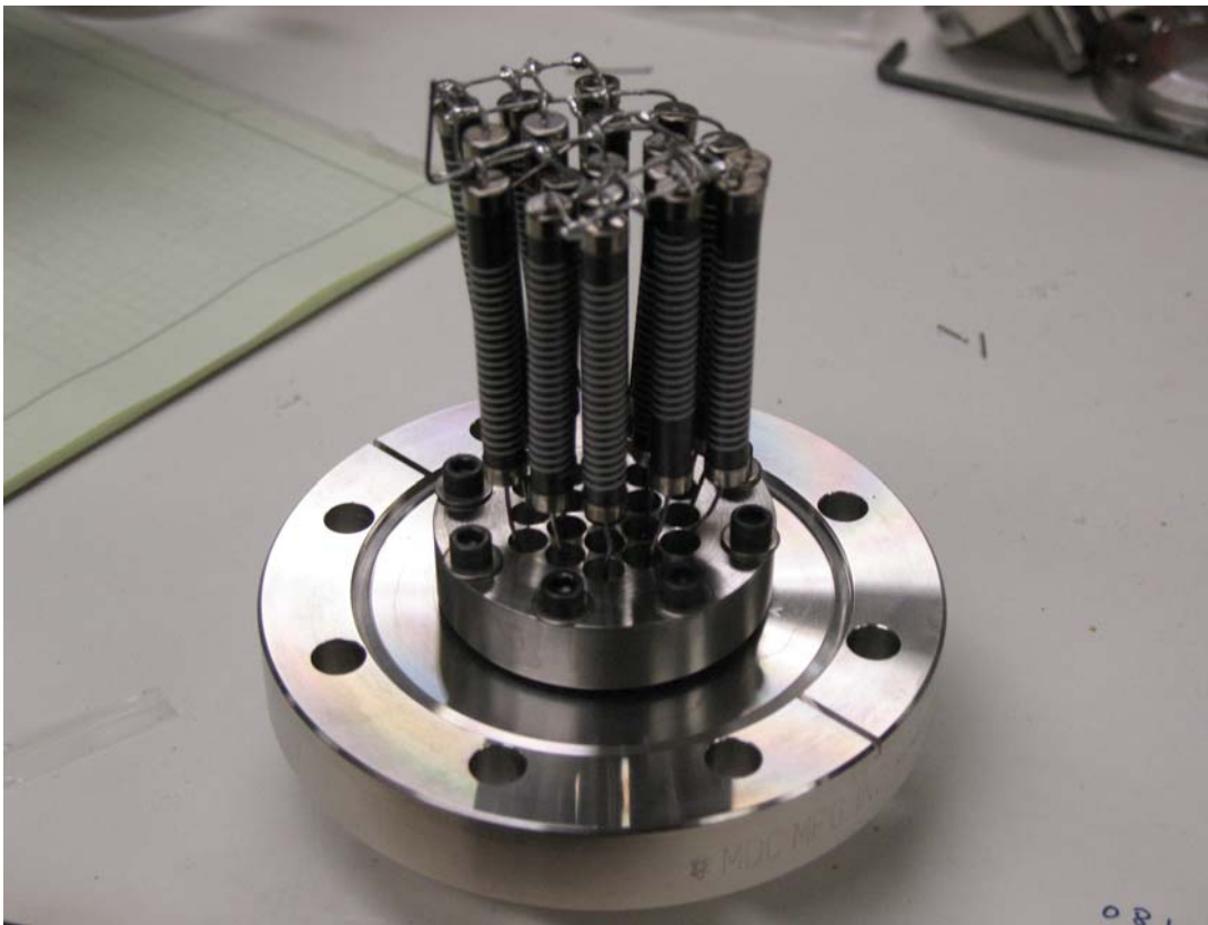
Figure 4 4 Megohm 4 watt Cermet film vacuum compatible resistors manufactured by Dale-Vishay for mercury and sodium vapor lamps. The resistors are fed from a common source and are in series with the individual needles. The resistors can dissipate about 4 watts each when cooled by the nitrogen flow.
