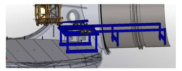
5.1.8 Attach the "Rail, ACB Assembly" (D1101724) to the "Suspension Lift Assembly" (D1101953) using two SHCS (¼-20 x .62").
