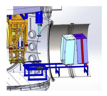
5.3.5 The **Slide Assembly** feet have Teflon pads that allow for an easy slide down the rail. There are blocks attached to the end of the rails to prevent travel past the **Table** end. Slide the **Baffle Box** toward the QUAD until it is positioned directly above the **Wedge Lift**,
