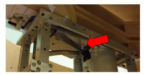
5.2.16 Remove four 1/4-20 SHCS and "SIDE BEAM" (D1102026) from Installation Stand on the side closest to the chamber wall. Remove from vacuum system.
