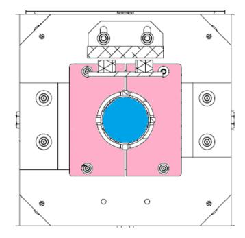
2.3.6 When balancing is complete, re-attach the **Transport Locking Bracket**.
