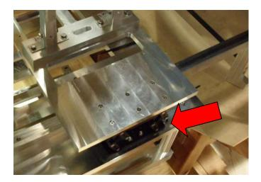
5.2.13 The two people on each side of the **Table** uniformly raise the **Jacks** to lift the **Installation Stand** and align **Interface Mounting Plate** to **STAGE-0** mounting locations. Continue until top of **Interface Mounting Plate** touches **STAGE-0**.
