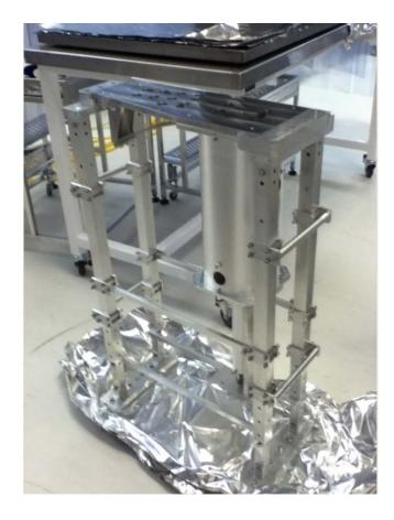
7 - Replace and fasten the **Upper Clamp** and the **Side Beams** with the saved hardware.
