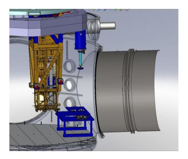
5.2.23 Remove the twelve 1/4-20 SHCS attaching the **Secondary Table** to the **Suspension Lift Assembly**. Place SHCS on aluminum foil container in bottom of spool for use in next step.
