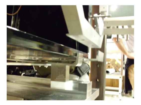
5.3.10 Pull **Slide Assembly** along **Rail Assembly** to end toward spool, and leave it there until later removing through the manifold tube.
