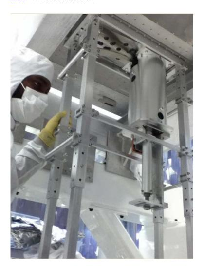
2.1.10 Remove **Side Beam** from **Installation Stand** from each side one at a time, clamping that side with **Dog Clamps** before removing the other side. Remove parts and set aside.
