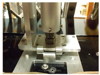
5.3.7 Attach **Baffle Box Assembly** to **Suspension Assembly** with one #10-24 Shoulder Screw (D1101293), three #10 Flat Washers, and one #10 Silver Plated Nut
