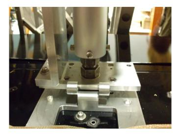
2.2.8 Attach **Baffle Box Assembly** to **Suspension Assembly** with **Shoulder Screw** (D1101293), three #10 Flat Washers, and one #10 Silver Plated Nut
