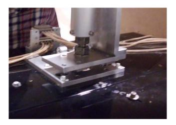
5.3.6 The two people on each side of the **Table** uniformly raise the **Jacks** to lift **Baffle Box Assembly** and align to top hinge plate at bottom of **Suspension Assembly**. Adjust **Baffle Box** position as needed for alignment. Continue lifting until hinge plates touch.
