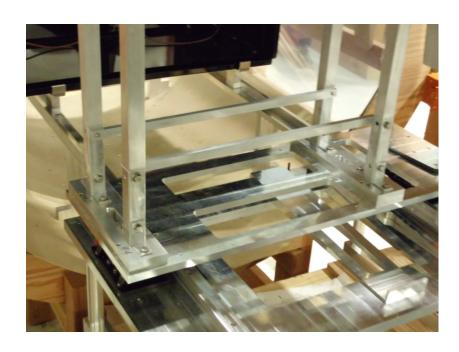
5.2.3 The two people inside the chamber will adjust the **Table, Secondary, Suspension**" (D1101962) so that it is directly below the Stage 0 position where the ACB suspension will be attached.
