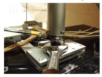
5.5.20 When correct height is obtained, tighten the SHCS of the **Variable Bracket Assembly** in the slotted holes.
