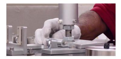
5.3.8 Attach four SHCS (1/4-20 x 7/8") through **Top Hinge Plate on Suspension Ass**embly to **Bottom Hinge Plate** on **Baffle Box Assembly**.
