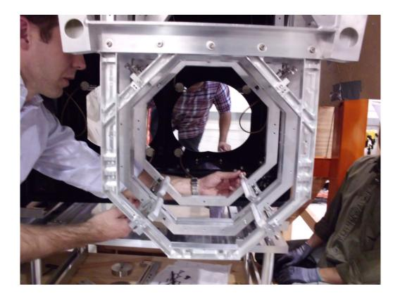
5.3.11 Detach Rail Assembly from Table and store in the manifold for later removal from vacuum system.
