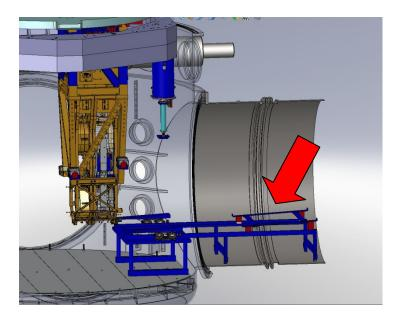
5.3.4 Using the "Slide, Baffle Carrier Assembly" (D1101958) and the "sedan chair" rods to lift the "Arm Cavity Baffle Box Assembly" (D1000977), which is stored in the manifold, two people will carry it and place the Slide, Baffle Carrier Assembly (supporting the baffle box) into the guides on top of "Rail, ACB Assembly" (D1101724); one person will be positioned in the spool behind the Baffle Box and another in front of the baffle box. The Baffle Box weighs about 100 lbs.
