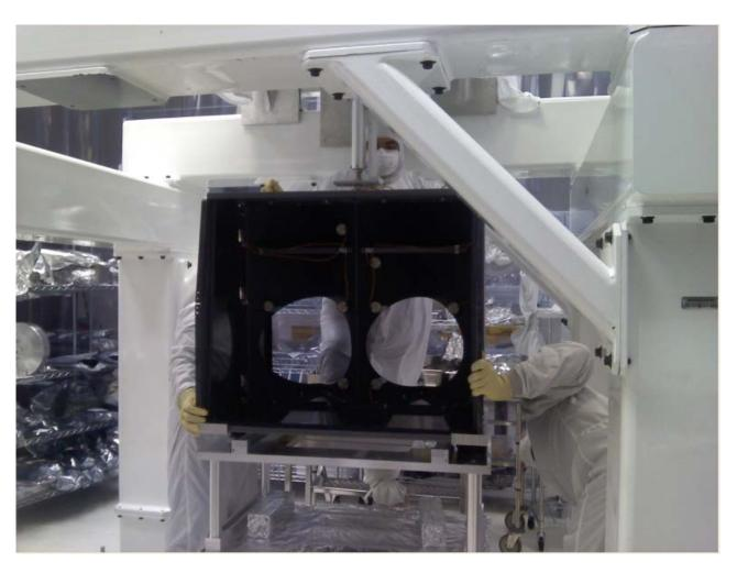
2.2.7 Crank lifting Table (D1002192) upwards to lift Baffle Box Assembly and align to Top Hinge Plate at bottom of Suspension Assembly. Adjust Baffle Box position by moving the cranked lower lifting table as needed for alignment. Continue lift until plates touch.
