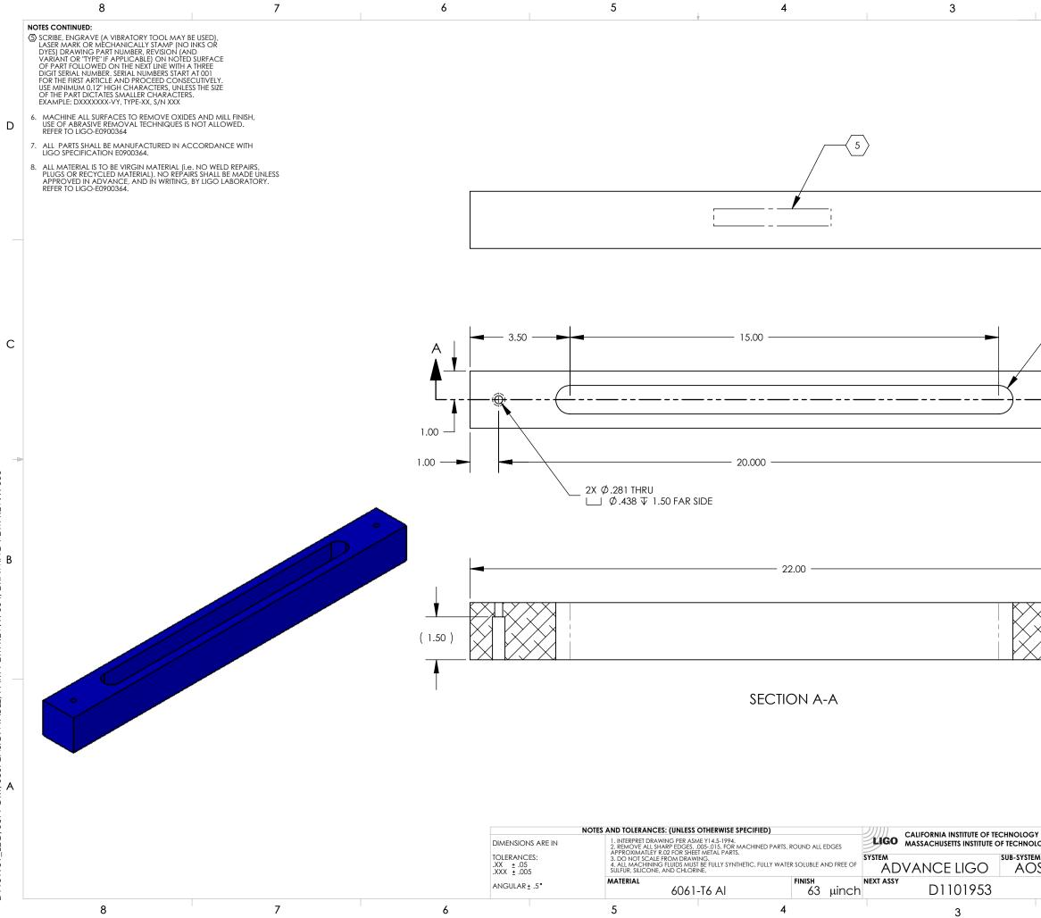
D1101951\_LEG, SUPPORT, SUSPENSION TABLE, PART PDM REV: X-004, DRAWING PDM REV: X-006
