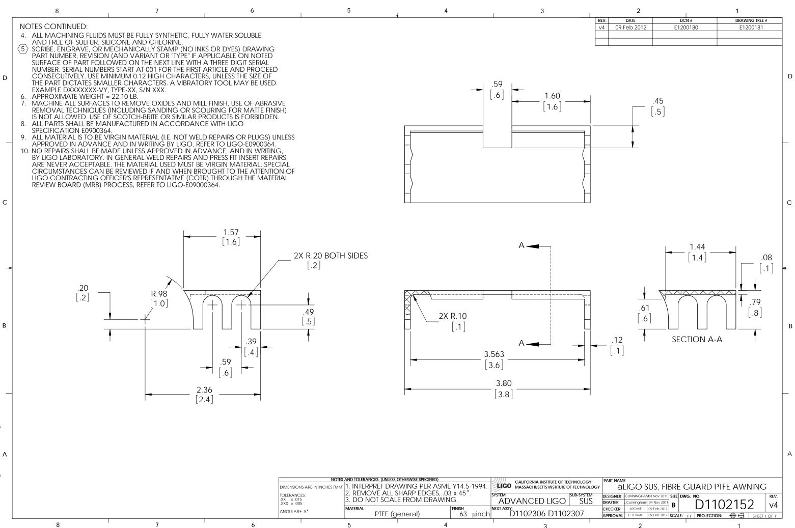
PART PDM REV: X-002, DRAWING PDM REV: X-001
