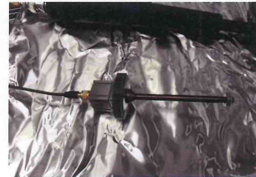
Figure 2: Custom Accelerometer Mount
