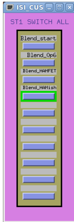
Figure 4: The SWITCH ALL blend screen, which simultaneously switches all the DOF to the selected blend.
