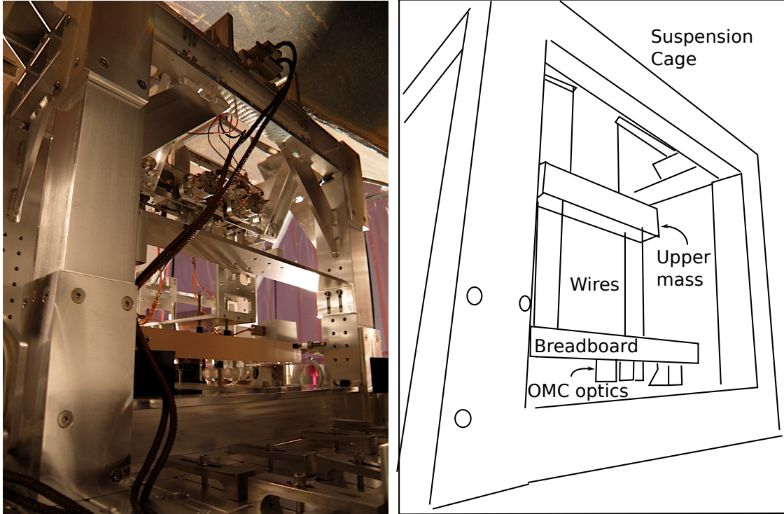
Figure 3-5: Photograph of the OMC double pendulum suspension. The line sketch shows the upper mass stage, which is obscured in the photograph by the coil actuators.
